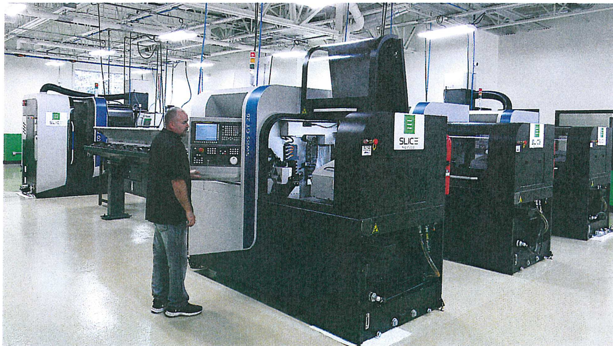
Brad Fowler, Manufacturing Technologist at Slice Mfg. Studios - wide view of 3 Swiss GT 26 machines.
