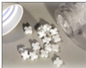
Figure 2. The implant device was composed of multiple ceramic crosses (5x5x3mm).
